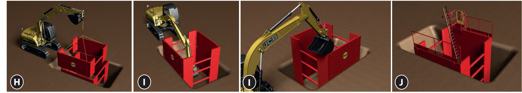
H Lower Top onto Base and connect together to form single box ensuring all 4 top to base connection points are fully secured I Dig and push assembled box to box depth / required depth. If additional top required repeat steps H to I J On reaching final depth batter back open ends. Install MGF ladder and edge protection. NB. Endsafe panels or trench sheets can be used in lieu of a batter
